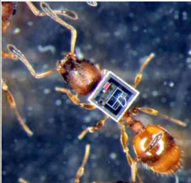
Commercialized IC for specimen tagging purposes [1]
